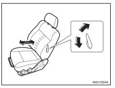
To adjust the front seat lumbar support, use the lever located on the outboard side of the seatback.
